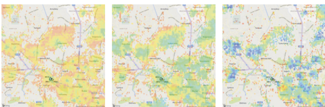
Geo-located customer experience (signal strength/quality and too many server) maps, created for single site verification
