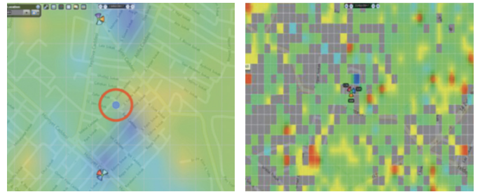
Geo-located customer experience (blended and high-res discrete, signal strength) maps for customer complaints analysis
